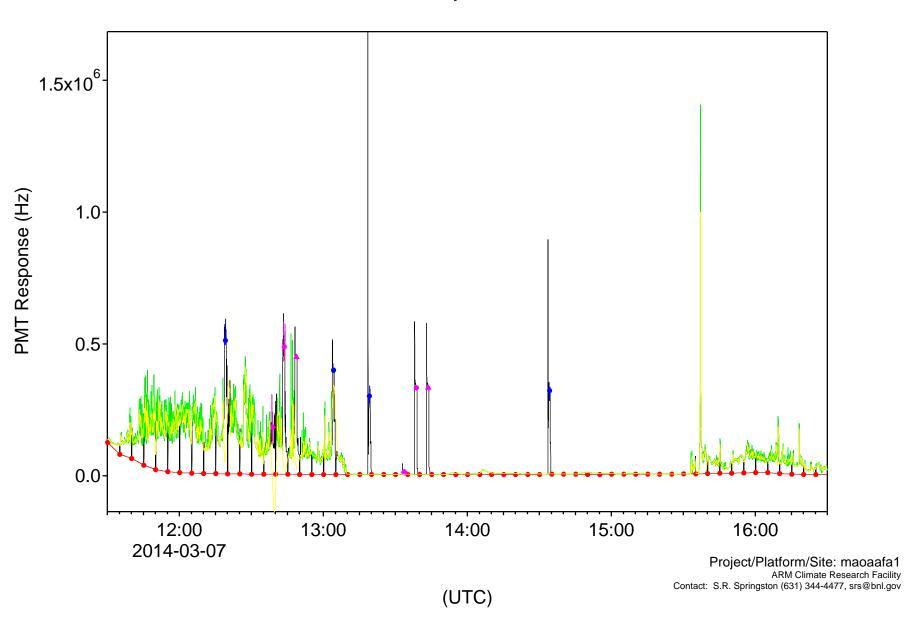
AAF 3-Channel NO<sub>x</sub> Analyzer Parsed NOx Channel Data
