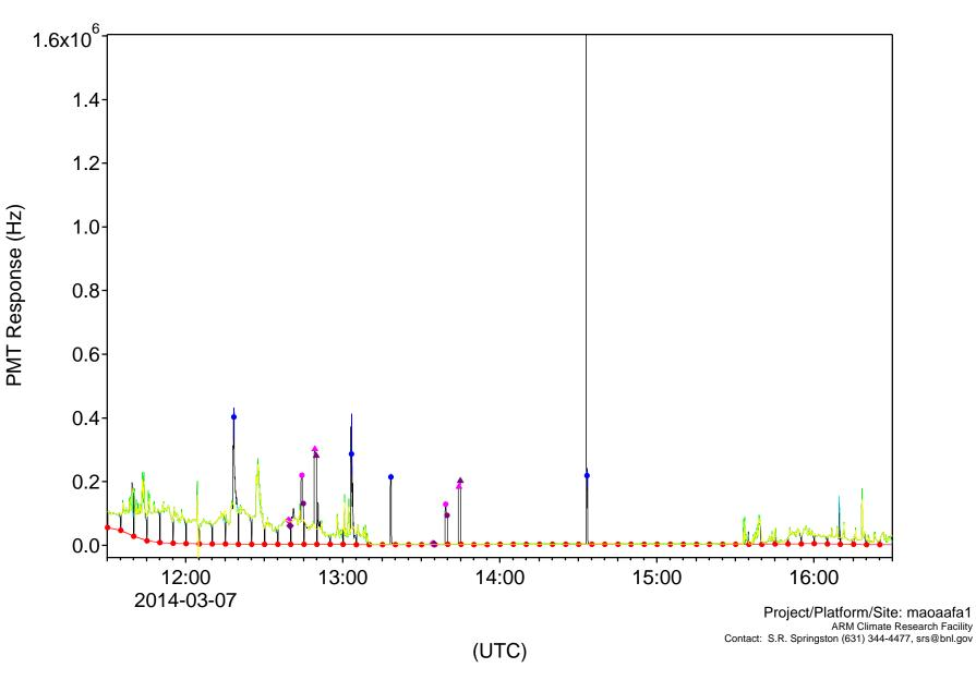
AAF 3-Channel NO<sub>x</sub> Analyzer Parsed NO Channel Data
