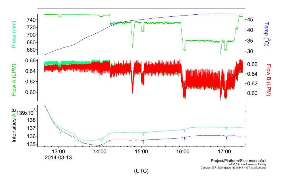
TEI Model 49i UV Photometric Ozone Analyzer Zero/Span Checks
