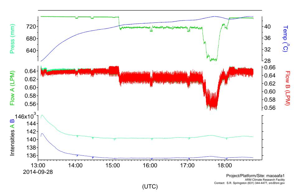
TEI Model 49i UV Photometric Ozone Analyzer Housekeeping TEI Model 49i UV Photometric Ozone Analyzer Zero/Span Checks
