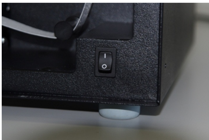
Figure 8. Power on switches: rear panel (top) and inside the door on the right (bottom).
