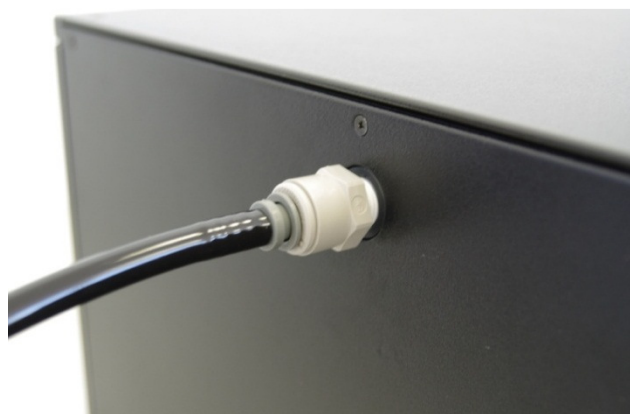
Figure 7. Fit the inlet connector on the rear panel of the Aethalometer and connect the sampling line tubing to it.
