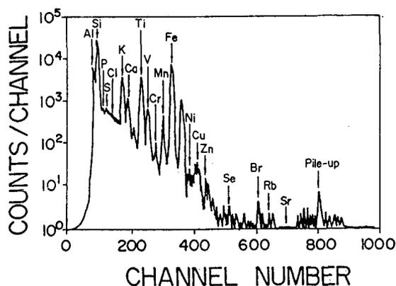
Fig. 2. A typical PIXE spectrum of a soil sample from the Pindorama's Experimental Station.
