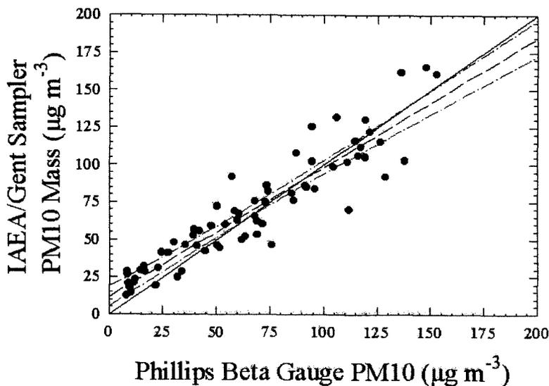
FIGURE 7. Comparison of  $\text{PM}_{10}$  ( $\mu\text{g m}^{-3}$ ) measured with an IAEA/Gent SFU sampler and a Phillips  $\text{PM}_{10}$  inlet beta gauge.
