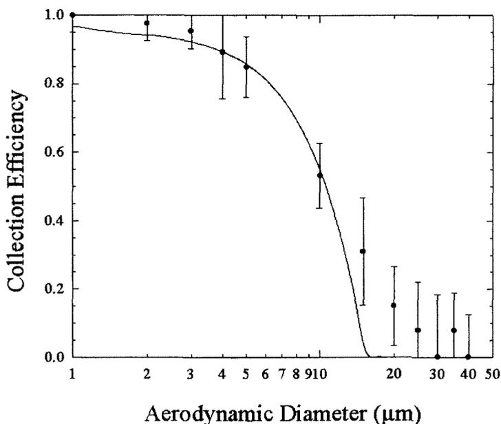
FIGURE 3. Collection efficiency as a function of aerodynamic diameter after applying the wall loss corrections. The error bars are the standard deviation of the 11 inlet samples. The line is the theoretical PM<sub>10</sub> sampler efficiency as defined by the U.S. Environmental Protection Agency.
