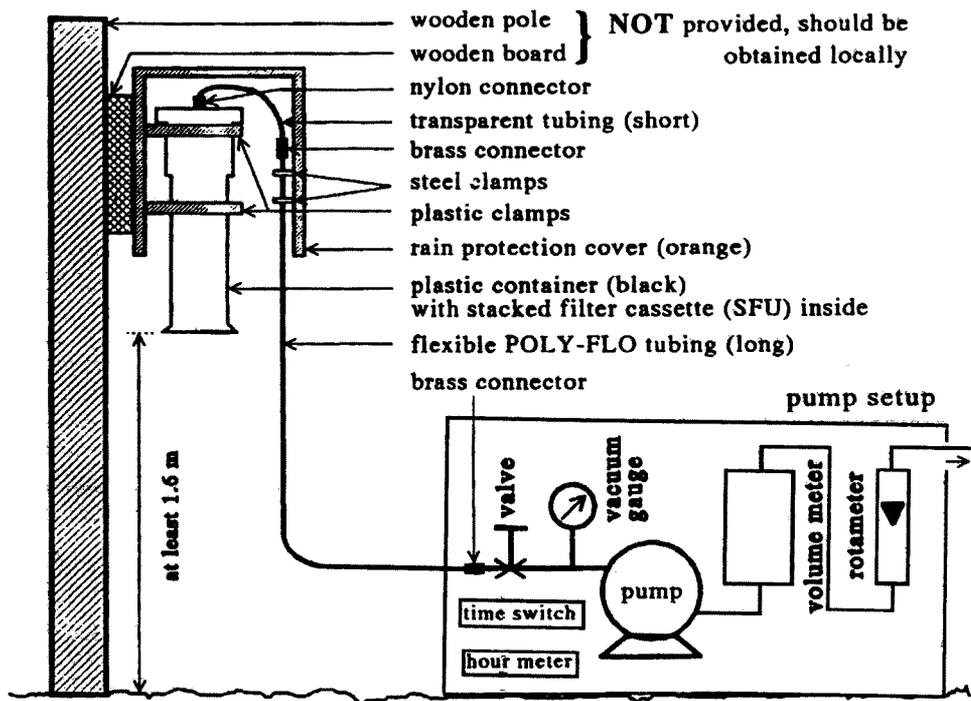
FIGURE 2. Schematic of the sampling system as typically deployed in the field including the pump, flow control system, and rain shield.
