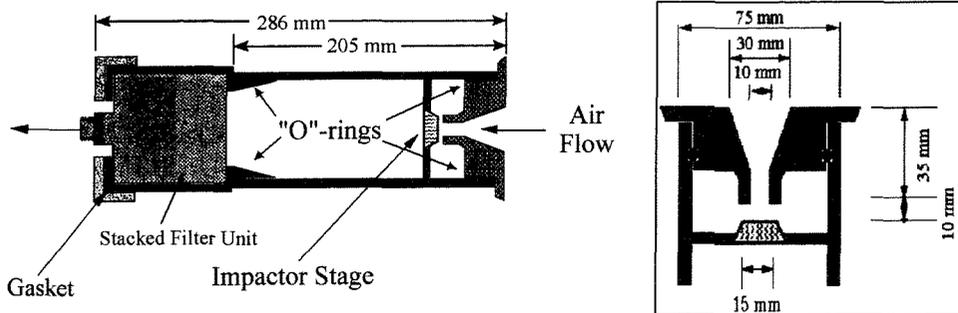
FIGURE 1. Schematic of the sampling head containing the  $10 \mu\text{m}$  impactor inlet and the NILU SFU.
