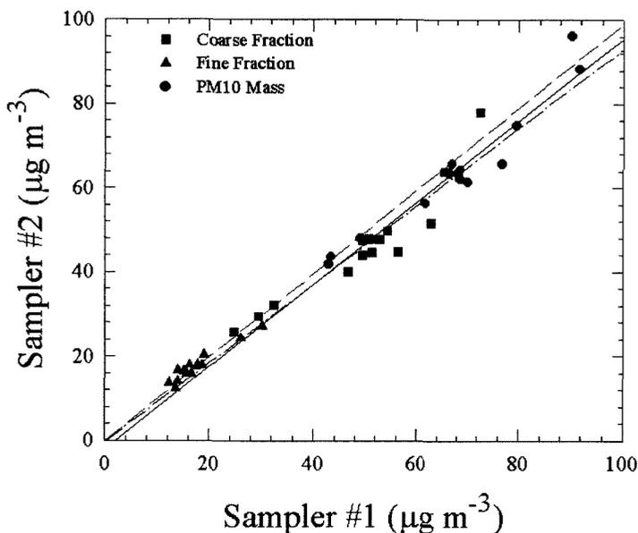
FIGURE 5. Comparison of the coarse fraction mass ( $\mu g m^{-3}$ ) [top], fine fraction mass ( $\mu g m^{-3}$ ) [middle] and total  $PM_{10}$  mass ( $\mu g m^{-3}$ ) [bottom] for side-by-side samplers using  $0.4 \mu m$  pore Nuclepore® filters as the fine fraction filters.
