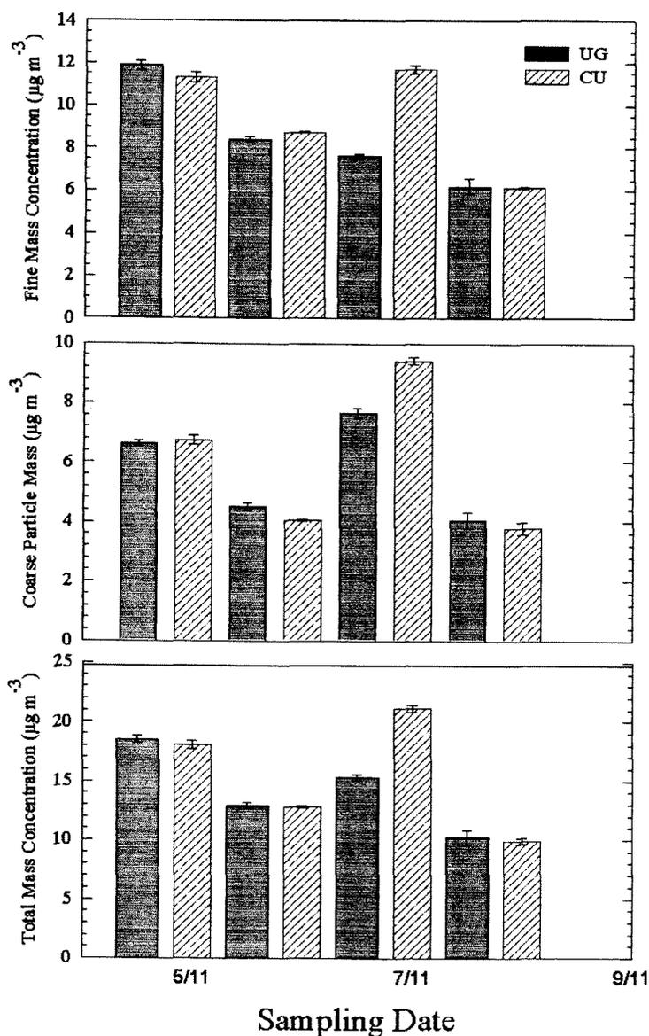
FIGURE 4. Comparison of the fine fraction mass ( $ng m^{-3}$ ) [top], the coarse fraction mass ( $ng m^{-3}$ ) [middle] and the total mass  $ng m^{-3}$  [bottom] for the two side-by-side samples manufactured in different laboratories.
