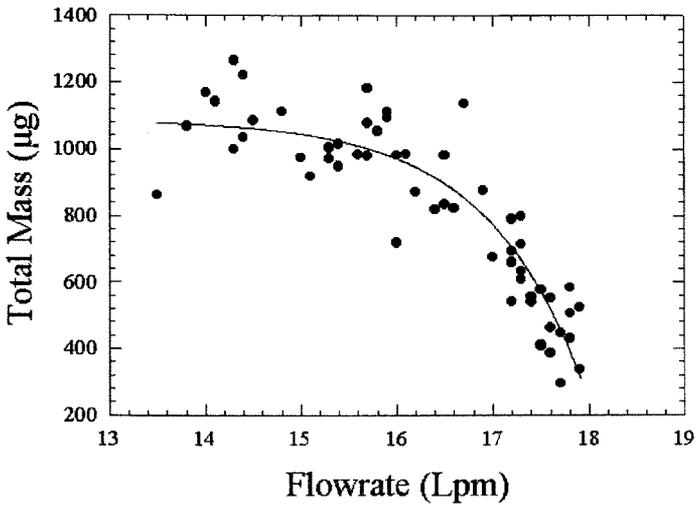
FIGURE 9. The effect of total mass collected in the SFU (fine plus coarse) on the flowrate through the IAEA/Gent SFU sampler.
