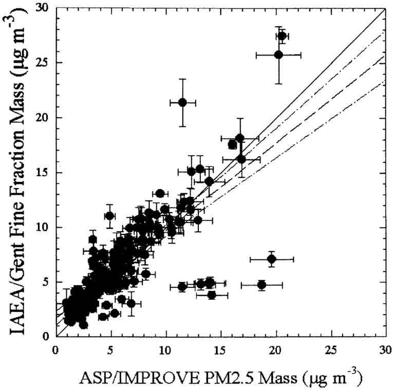
FIGURE 8. Comparison of fine particle mass ( $< 2.5 \mu\text{g m}^{-3}$ ) measured with an IAEA/Gent SFU sampler and an ASP/IMPROVE cyclone sampler.
