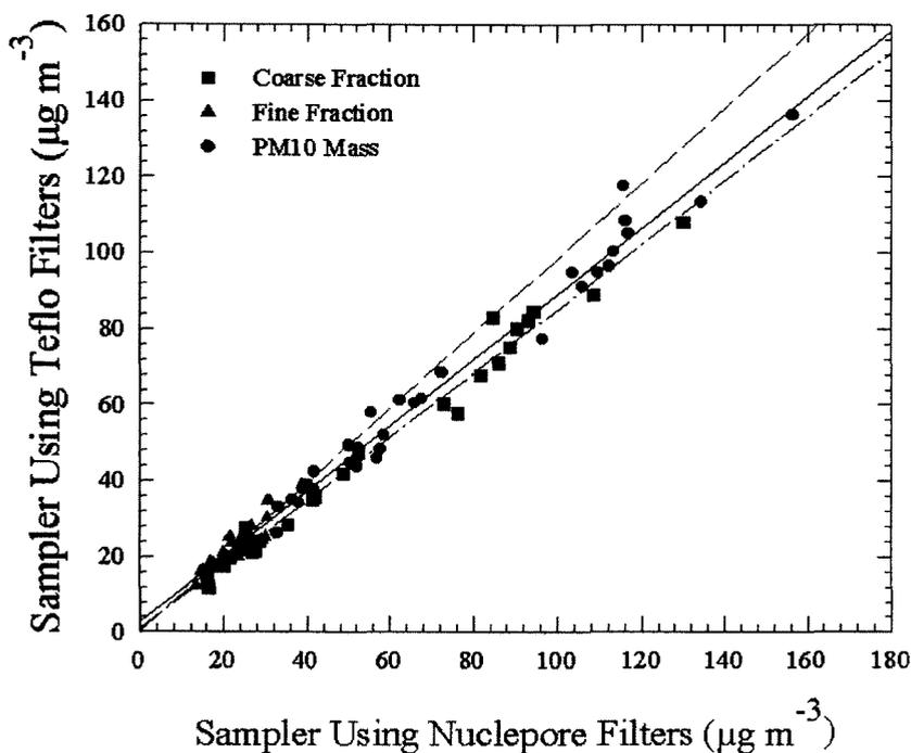
FIGURE 6. Comparison of the coarse fraction mass ( $\mu\text{g m}^{-3}$ ) [top], fine fraction mass ( $\mu\text{g m}^{-3}$ ) [middle] and total  $\text{PM}_{10}$  mass ( $\mu\text{g m}^{-3}$ ) [bottom] for side-by-side samplers using a  $0.4 \mu\text{m}$  pore Nuclepore<sup>®</sup> and a  $2 \mu\text{m}$  pore Teflo<sup>®</sup> filter as the fine fraction filters.
