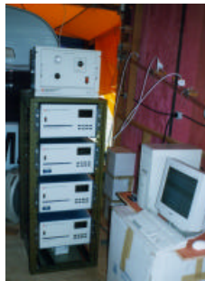
Figure 6- Real time Monitors of O 3 , NO x e CO of Thermo Environmental Instruments.
