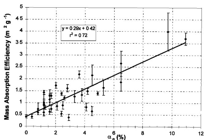
**Figure 4.** Nonsphericity parameter ( $\alpha_o$ ) versus the total mass absorption efficiency ( $\alpha_a$ ). Nonspherical particles and clusters are associated with high values of  $\alpha_a$  and high ratios of black carbon (BC) mass to total particle mass (TPM).
