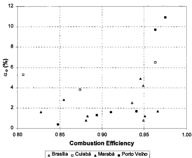
**Figure 3.** Nonsphericity parameter ( $\alpha_o$ ) versus combustion efficiency. More asymmetrical particles and clusters are generally associated with higher combustion efficiency (flaming-phase combustion).
