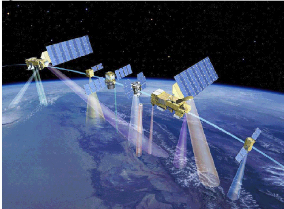
Figure 7-7. The A train – a constellation of satellites that jointly will measure aerosol, clouds and precipitation properties.
