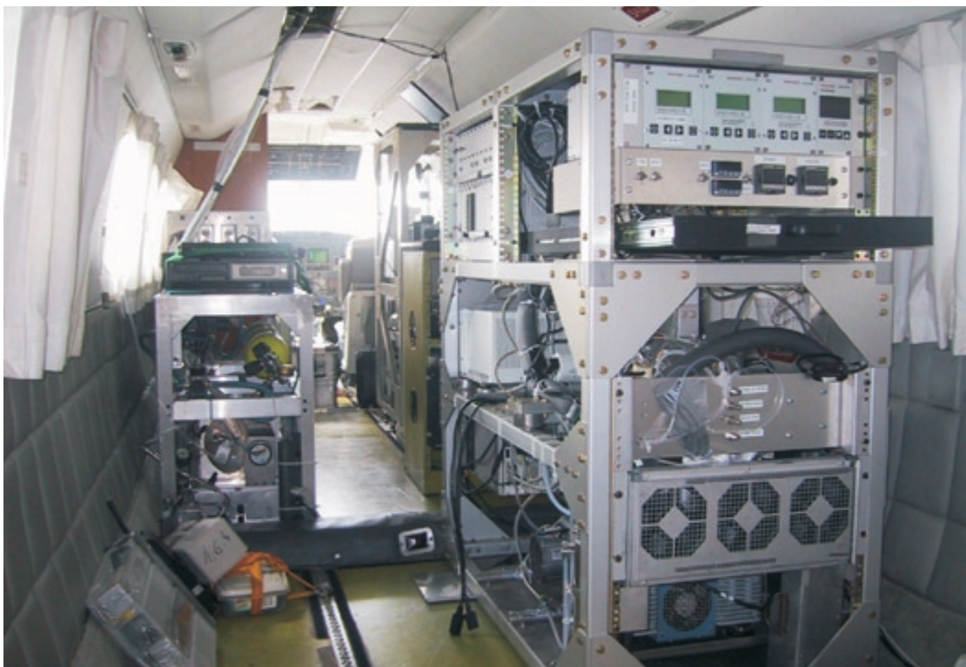
Figure 2. Instrumentation used in TROFFEE on the INPE Bandeirante aircraft: on the right PTR-MS (NCAR) and on the left Airborne FTIR and whole air sampling (University of Montana and University of California Irvine). In front O 3 , PM 10 , 3-wavelength nephelometry, GPS (University of São Paulo).
