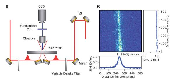
**Fig. 1** (A) Crossed-beam SHG microscope for a kHz amplifier laser producing 120 fs pulses operating at incident angles of 20° from the surface normal. The SHG response is imaged at normal incidence. (B) Background subtracted SHG image obtained from a plain glass slide at 400 nm. The horizontal and vertical profiles of the SHG E-field, normalized to its highest value and referenced to zero, and Gaussian fit on the horizontal profile.
