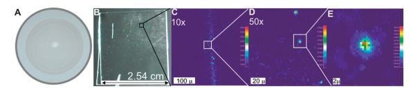
**Fig. 3** Optical images of (A) MOUDI stage 3 collector plate  $(3.2-5.6 \,\mu\text{m}$  size range; aerodynamic diameter) and (B) a  $1 \times 1$  square inch glass slide onto which the filter had been pressed. SHG images obtained with a  $10 \times (C)$  and  $50 \times (D)$  objective from the area marked by the square. (E) View of the SHG image shown in (D), zoomed to the rectangular area.
