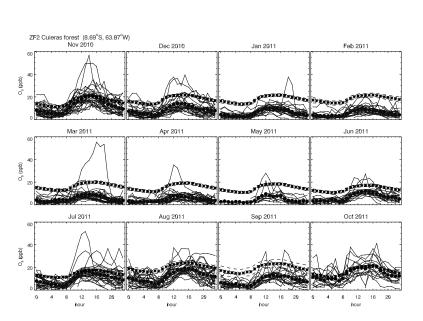
**Figure 2.** Comparison of measured and simulated monthly averaged diurnal cycle of surface  $O_3$  mixing ratios at the ZF2 site in the Cuieiras forest reserve, including measured day-to-day variability and standard deviation for the model results. The measurements have an uncertainty of 4%. We show one of the two available years of observations. Legend as in Fig. 1.
