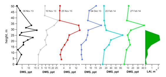
**Figure 6.** Example of high vertically resolved DMS mixing ratio measurements by GC-MS during the afternoon (13:00–15:00) on the K34 tower made between November 2013 and February 2014. Also shown are vertically resolved measurements of leaf area index (LAI). Note the buildup of DMS near the top and just above the 30 m canopy with mixing ratios up to 80 ppt.
