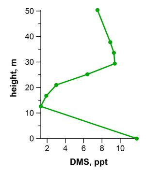
**Figure 7.** Example of high vertically resolved DMS mixing ratio measurements by GC-MS approximately 30 min following a rainstorm in the afternoon (14:06–14:55) on the K34 tower. Note that in addition to the buildup of DMS within the canopy, a buildup near the surface was observed, suggesting a potential increase in soil emissions as a result of wetting.
