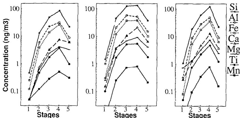
Fig. 3. Elemental size distribution for biogenic related elements at the three levels of the Ducke Reserve Tower (left: ground level, middle: canopy level, right: top level). The 50% cutoff diameters for the cascade impactor stages 1, 2, 3, 4, and 5 are 0.25, 0.5, 1, 2 and 4  $\mu\text{m}$ , respectively.
