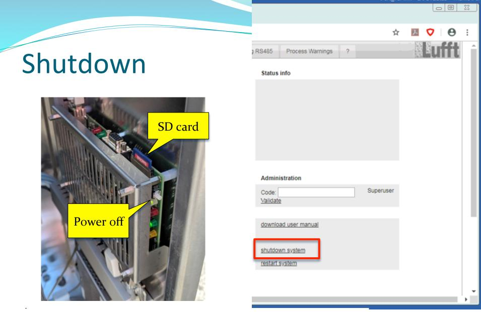
2. Service trained persons may also open the inner housing door and press the white "shut down" button at the main controller (check service manual for details)
