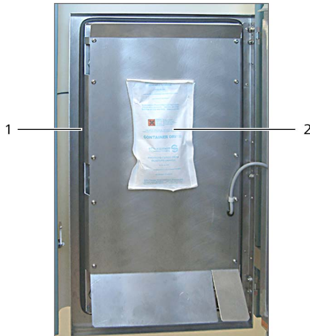
Fig. 28: Air dehumidifier bag (2) and rubber seal (1).
