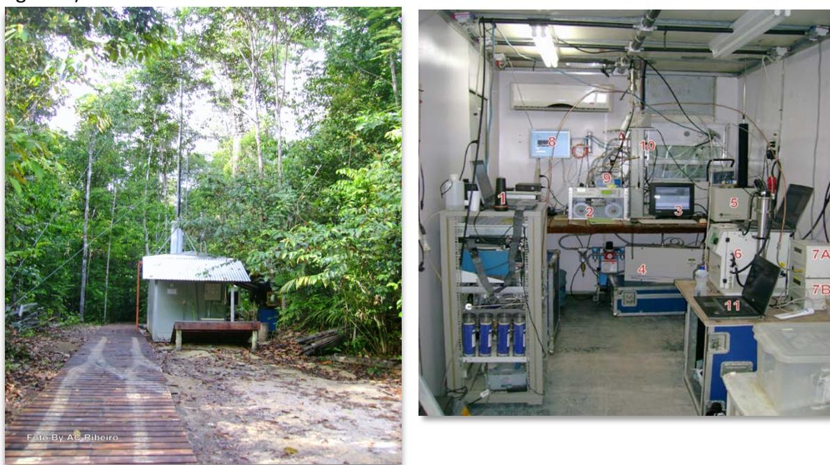
**Figure 8** - External view of the atmospheric observation container in operation at the TT34 site. The container has air conditioning and a large dryer to allow dry sampling conditions for aerosol (left). On the right picture we can see an internal view of the container with several instruments in operation. The site operates continuously from February 2008, as part of the FAPESP Thematic Project AEROCLIMA.
